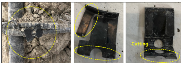
(b) Failure mode of the initial clip-type binding implement
